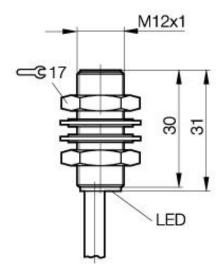
Inductive Sensors BES 516-325-G-E4-Y-PU-05 M12x1 x 31 normally-open Sn=4mm shielded
